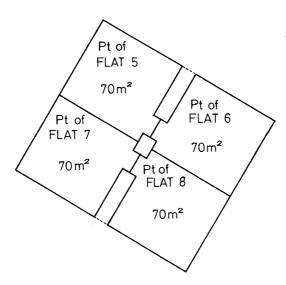
HORIZONTAL BOUNDARIES OF FLATS ARE DEFINED BY HEAVY BLACK LINES BOUNDARIES OF FLATS ARE THE CENTRE OF FLOORS WALLS AND CEILINGS UNLESS OTHERWISE DEFINED PORTIONS OF FLATS WITH HORIZONTAL BOUNDARIES DEFINED BY DIMENSIONS ARE OPEN SARPORTS AND THE VERTICAL BOUNDARIES EXTEND FROM GROUND LEVEL TO THE UNDERSIDE OF THE ROOF AREAS SHOWN ARE TOTAL AREA OF THE FLATS.
