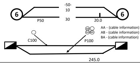
One 50mm PVC conduit (P50) containing a 50-pair and a 10-pair cable between two 6-pits. approximately 20.0m apart, with a direct buried 30-pair cable along the same route
