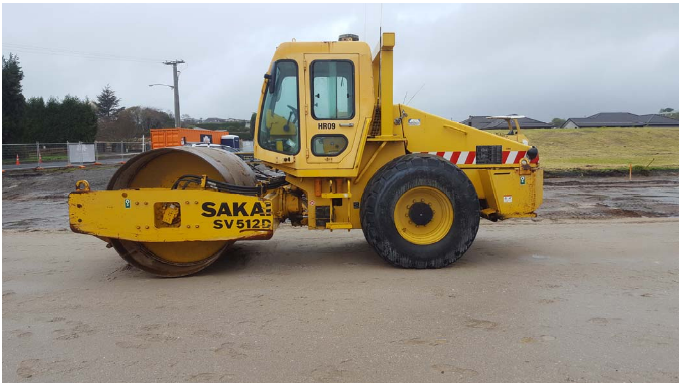
Figure 4: 10T roller used.
